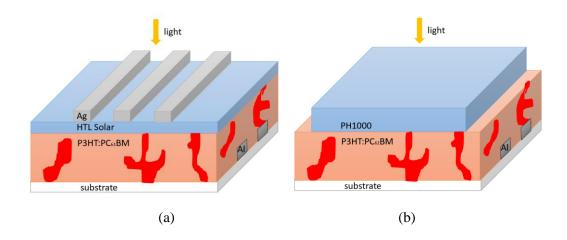
Figure 3.14. Transparent top electrode inverted solar cell designs. In (a) the anode is made of a thin layer of silver over an HTL, while in (b) PH1000 serves as both the HTL and anode. In both cases, the cathodes (visible on the right side of the solar cells) and the anodes are perpendicular in order to create several small area solar cells per sample.
