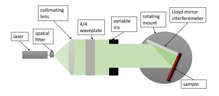
Figure 2.35. Top-view schematic of grating inscription set-up. A lens collimates the laser beam, which is then circularly polarized before irradiating the Lloyd's mirror interferometer.
