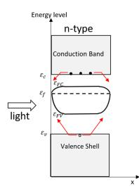
Figure 2.8. Quasi-Fermi levels in a n-type material, where  $\varepsilon_c$  and  $\varepsilon_v$  are the energy level of the conduction band and valence shell, respectively. The gradients of the quasi-Fermi levels  $\varepsilon_{FC}$  and  $\varepsilon_{FV}$  drive the electrons and holes toward the surfaces. However, as the material is symmetrical, there is no preferential path for the carriers and therefore no current.
