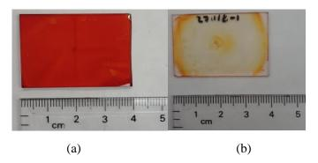
Figure 3.22. Azobenzene thin film (a) before and (b) after a 20-hour UV exposure.
