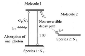
Figure 2.42. Model for the photodegradation process of azobenzene molecules. Initial molecules are raised to the *cis* excited state be means of absorption of a photon, but decay to new species instead of relaxing back to their *trans* ground state, making the process irreversible. Adapted from (Galvan-Gonzalez *et al.*, 2000)<sup>147</sup>.
