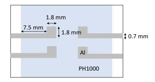
Figure 3.12. Schematic of the electrodes patterning of Al/PH1000 solar cells. To minimise the increase in the solar cell's series resistance, the aluminum was the electrode chosen for patterning.
