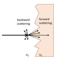
Figure 2.37. Backward and forward scattering of incident light at the interface of a rough surface.
