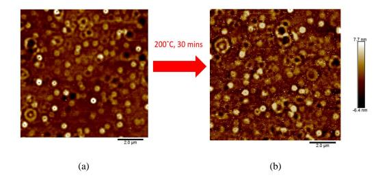
Figure 4.20. 2D profile of a UV treated azobenzene thin film (a) before and (b) after being heated at 200°C for 30 minutes. The high temperature exposure had no apparent effect on the volcano-like nanostructures.
