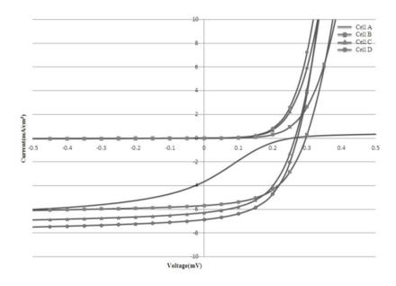
Figure 2.24. Effect of interfacial layers between the active layer and the cathode in a direct structure solar cell. Cell A is a reference device, Cell B, C, and D include respectively interfacial layers of Ca, BCP, and BCP + Ca. Adapted from (Kim *et al.*, 2010)<sup>120</sup>.
