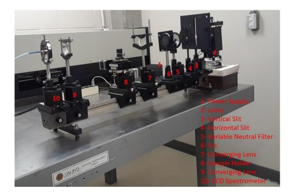
Figure 3.4. Spectrometry set-up #1. This set-up can be used to measure the transmission and absorption of thin films in the 300-1000 nm wavelength range.
