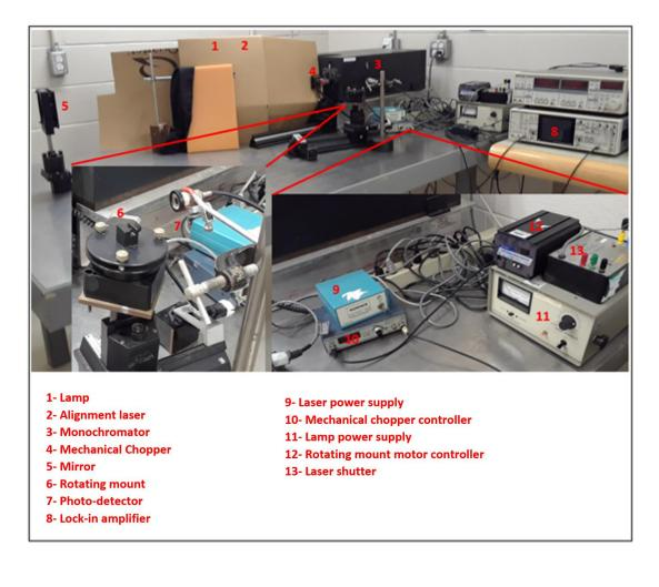
Figure 3.5. Spectrometry set-up #2. The source is provided by a halogen lamp (behind the cardboard in the picture). The light is then split by a monochromator before being reflected on the sample. A laser (also behind the cardboard in the picture) is used for sample alignment. Two insets give a closer look at the equipment # 6-13.
