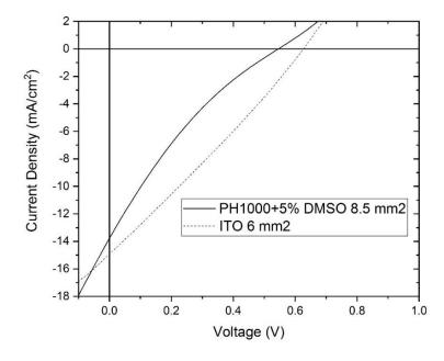
Figure 4.9. J-V characteristic curves of direct structure solar cells with ITO and PH1000 bottom electrodes. Though the PH1000-based solar cell shows a lower FF and current density, PH100 electrode remains an acceptable alternative to ITO.
