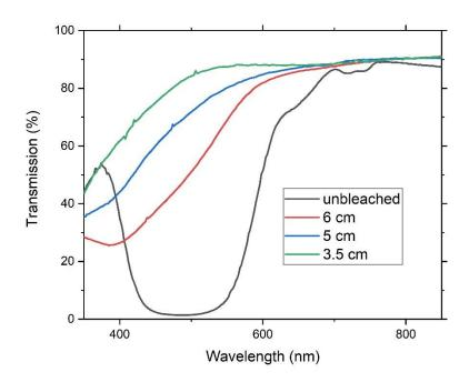
Figure 4.29. Transmission of patterned azobenzene thin films after a 20-hour UV exposure at different distance from the UV lamp. The films achieved a better transmission at a closer distance from the lamp.
