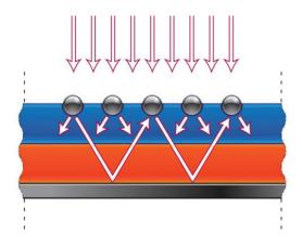
Figure 1.6. Metal nanoparticles acting as scattering centers in a thin film solar cell. The nanoparticles also act as top reflectors for the light reflected by the bottom electrode. Adapted from (Atwater and Polman, 2010)<sup>36</sup>.
