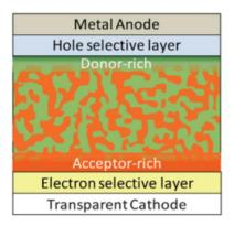
Figure 2.19. Schematic illustration of the vertical separation of a polymer:fullerene blend in an inverted solar cell. The fullerene, the electron acceptor, concentrates at the bottom of the cell during film formation. The inverted cell structure, with a bottom cathode, can therefore exploit this phase separation. Adapted from (Yip and Jen, 2012)<sup>75</sup>.
