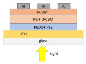
Figure 3.11. Schematic of an ITO solar cell with a  $PC_{61}BM$  over-layer. A thin layer of  $PC_{61}BM$  in DCM is deposited on top of a layer of P3HT:PC\_{61}BM in o-DCB.
