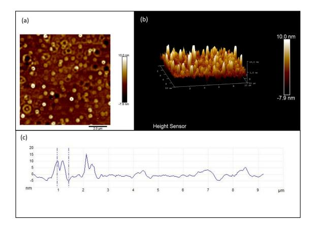
Figure 4.15. Nanostructures formation in as-cast azobenzene thin films exposed to UV light. Volcano-like nanostructures are shown in (a) 2D and (b) 3D with the profile shown in (c). The RMS roughness of the unbleached film was measured at  $R_q = 0.5$  nm with the maximum roughness  $R_{qmax} = 3$  nm. After UV light exposure, the roughness was increased to  $R_q = 2.1$  nm and  $R_{qmax} = 40$  nm.
