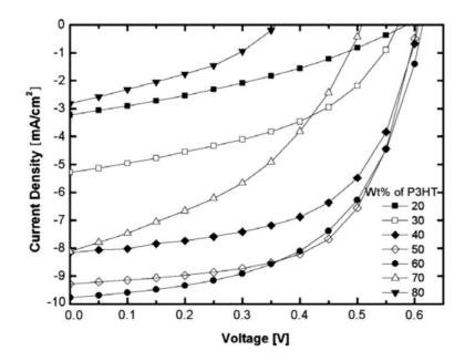
Figure 2.20. Effect of different ratios of P3HT:PC<sub>61</sub>BM blends on the J-V characteristic curve of a solar cell. Best results are achieved when P3HT:PCBM ratio of (1:0.8). Adapted from (Baek *et al.*, 2010)<sup>104</sup>.
