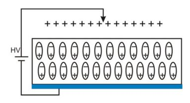
Figure 2.39. Schematic of a corona poling process. A high voltage is applied to an electrode, ionizing the surrounding air. This causes an alignment of the dipole in the material. Adapted from (Rahman, 2007)<sup>144</sup>.
