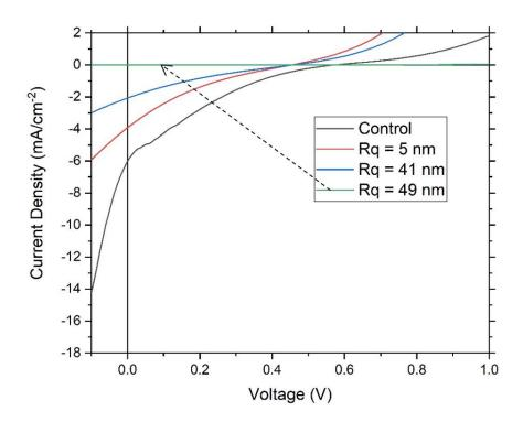
Figure 4.18. J-V characteristic curves of single-sided solar cells with azobenzene thin films patterned by corona poling. The efficiency of the solar cells quickly decreased with increasing values of  $R_q$ .
