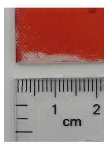
Figure 4.19. Damage on a gDR1 azobenzene thin film after curing at 120°C for 30 minutes.
