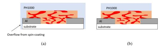
Figure 3.15. Overflow of PH1000 on the edges of a sample caused by spin-coating in (a) and clean edges in (b). Cleaning of the edges is a critical step to avoid short-circuiting the cell at the aluminum contact points.
