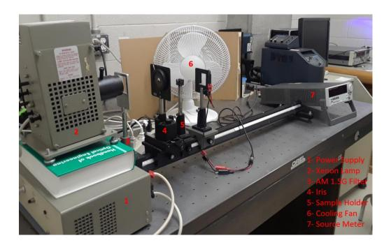
Figure 3.7. Solar cells characterization station. The combination of a xenon lamp with an AM1.5G filter closely matches the solar spectrum.
