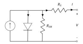
Figure 2.11. Equivalent circuit of a solar cell. A solar cell may be modelled by a current source in parallel with a diode, a shunt resistance and a series resistance.
