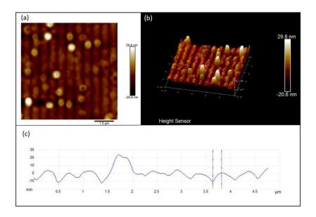
Figure 4.26. (a) 2D, (b) 3D and (c) profile of crossed grating on an azobenzene thin film after a 20-hour UV exposure. The UV exposure resulted in a partial destruction of the gratings and formation of volcano-like nanostructures.
