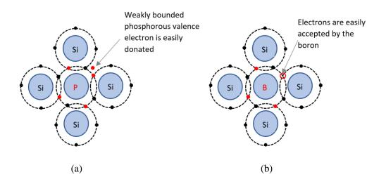
Figure 2.2. Doping of silicon with (a) phosphorus (n-type) and (b) boron (p-type). At non-absolute temperatures, the extra weakly bounded phosphorous valence electron in (a) is easily donated to the conduction band of a neighbouring silicon atom, while in (b) the holes in the lattice from the boron atom allow silicon electrons to move in the lattice.
