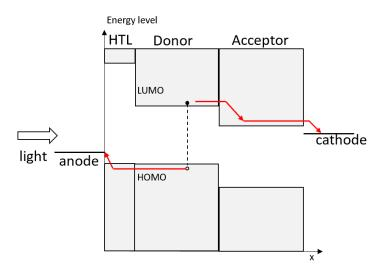
Figure 2.16. Energy levels in an organic polymer/fullerene solar cell. The absorption of photons generates excitons in the donor materials. The electrons are then funneled into a second material with lower LUMO level.
