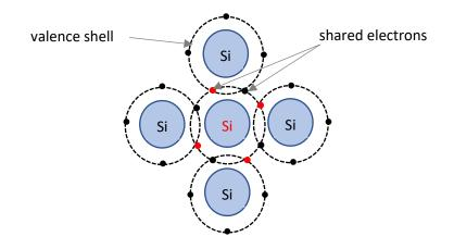
Figure 2.1. Pure silicon crystal lattice. Each silicon atom shares its valence electrons to form stable bonds with the neighbouring atoms.
