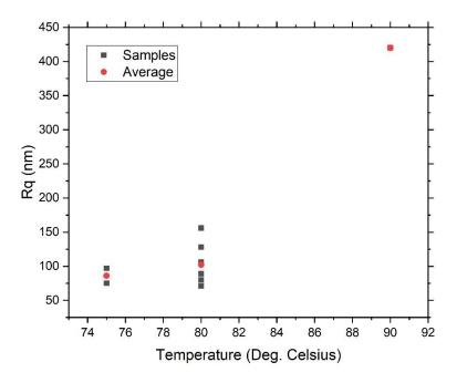
Figure 4.13. RMS roughness of corona-poled azobenzene thin films at different exposure temperatures. A higher exposure temperature resulted in an increase in  $R_q$ , with average values of  $R_q = 86$  nm,  $R_q = 102$  nm and  $R_q = 420$  nm for exposure temperature of 75°C, 80°C and 90°C respectively with a constant exposure time of 30 minutes and corona discharge voltage of 8 kV.
