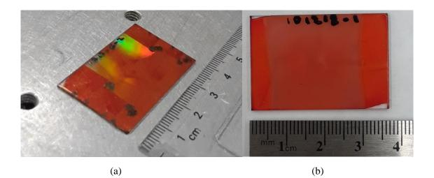
Figure 3.20. Azobenzene thin films patterned with (a) cross-gratings and (b) randomized nanostructures by corona poling.
