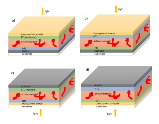
Figure 2.18. Architectures of bulk-heterojunction organic solar cells. Top illuminated solar cells are illustrated in a) with a direct structure and in b) with an inverted structure, while bottom illuminated solar cells are illustrated in c) with a direct structure and in d) with an inverted structure.
