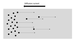
Figure 2.6. Diffusion current in a semiconductor. The electrons spread as a result of non-uniform concentration of charges. As the current is defined, by convention, as the direction of movement of a positive charge, the diffusion current is in the opposite direction of the movement of the electrons.
