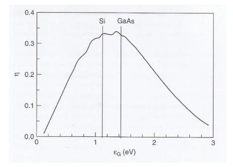
Figure 2.15. Efficiency  $\eta$  of a solar cell with radiation recombination only under AM1.5 as a function of bandgap. Adapted from (Würfel and Würfel, 2016)<sup>1</sup>.
