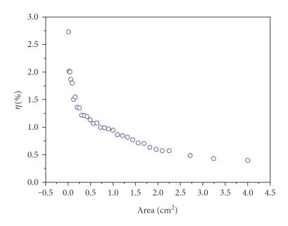
Figure 4.3. Area dependency of the efficiency of P3HT:PC<sub>61</sub>BM solar cells. Large area results in a sharp reduction of the efficiency. Adapted from (Trindade and Pereira, 2017)<sup>174</sup>.
