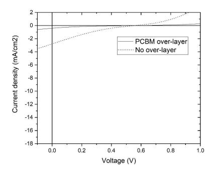
Figure 4.2. J-V characteristic curves of solar cells with and without a  $PC_{61}BM$  over-layer. The  $PC_{61}BM$  over-layer partially destroyed the under-layer, thus reducing the efficiency of the solar cell.
