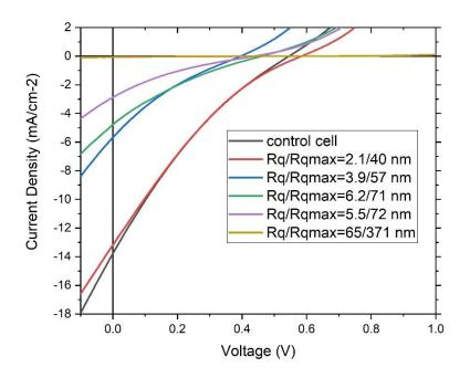
Figure 4.22. J-V characteristic curves for double-sided solar cells with azobenzene thin films patterned by corona poling and UV exposure. While the efficiencies of the solar cells showed some improvement with increased values of  $R_q$ , they quickly degraded with higher values of  $R_{qmax}$ .
