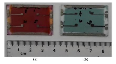
Figure 3.16. Image of (a) a P3HT:PC $_{61}$ BM and (b) a PTB7:PC $_{61}$ BM sample in a direct structure with PH1000 bottom electrodes. Each sample contains four solar cells.
