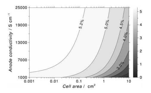
Figure 4.10. Effects of anode conductivity and solar cell area on the efficiency of P3HT:PC<sub>61</sub>BM solar cells. The efficiency of the cell decreases with lower conductivity and higher active area. Adapted from (Servaites *et al.*, 2010)<sup>77</sup>.
