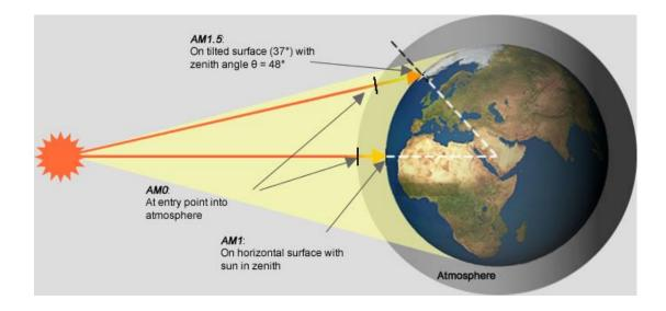
Figure 2.13. Length of the path through the atmosphere in relation to the shortest length for different solar spectrum. AM0 is typically used to test solar cells for spatial application, while AM1.5 is used to test solar cells for terrestrial application. Adapted from (Green Rhino Energy,  $2016)^{82}$ .
