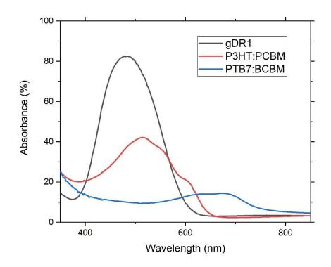
Figure 4.31. Absorbance spectra of thin films of gDR1, P3HT:PC<sub>61</sub>BM and PTB7:PC<sub>61</sub>BM. The azobenzene and P3HT:PC<sub>61</sub>BM absorbance spectra largely overlap.
