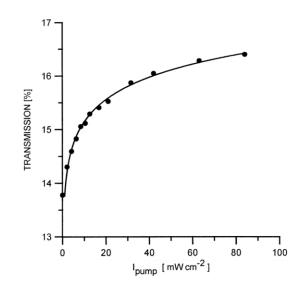
Figure 2.41. Transmission at a wavelength of 543.5 nm of azobenzene illuminated by a 532 nm laser. The transmission increases with the laser intensity. Adapted from (Miniewicz *et al.*, 1998)  $^{146}$ .
