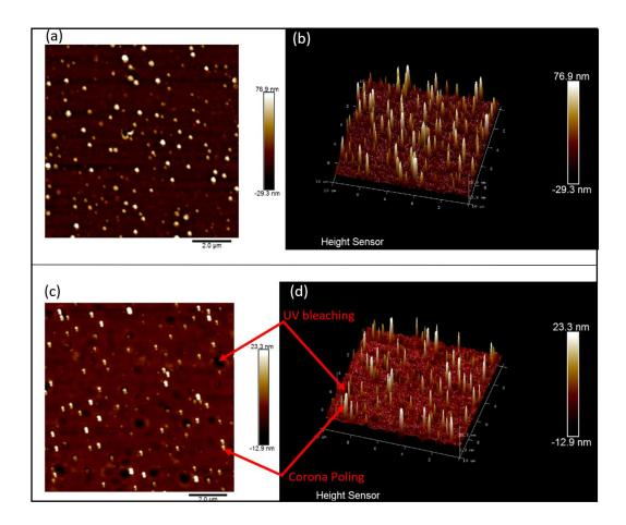
Figure 4.14. Formation of volcano-like nanostructures after UV treatment of a corona-poled azobenzene thin film. The 2D and 3D images of the untreated film are shown in (a) and (b) respectively, while (c) and (d) show the 2D and 3D images of the same film after a 20-hour UV exposure.
