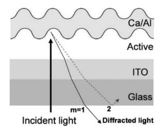
Figure 5.1. Schematic representation of the structure of a direct solar cell with a metal SRGs top electrode. The active layer is patterned by a PDMS mold before the evaporation of the top electrode. Adapted from (Na *et al.*, 2008)<sup>54</sup>.
