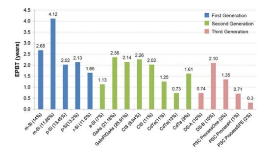
Figure 1.3. Energy payback time of selected solar cells. Within the third-generation solar cells, ProcessOne are indium-tin-oxide (ITO) based solar cells, ProcessH is ITO-free solar cells, and ProcessSFE is metal- and ITO-free solar cells. The efficiencies of the cells are indicated in brackets. Adapted from (Angmo *et al.*, 2014)<sup>13</sup>.
