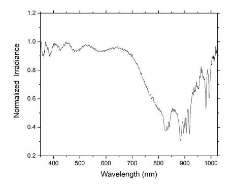
Figure 3.6. Normalized xenon arc lamp spectrum with an AM1.5G filter. The AM1.5G filter results in a reduction of the strong peaks of the xenon lamp in the near infra-red region to obtain a closer match with regards to the solar spectrum.
