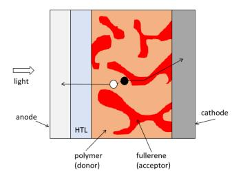
Figure 2.17. Charge separation in a bulk-heterojunction. Excitons are by the absorption of the photon energy in the polymer. Due to the reduced distance to the fullerene, the electrons can be funneled out before they recombined. A hole-transport layer provides a semi-permeable membrane, blocking the electrons from reaching the cathode.
