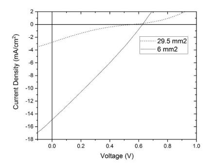
Figure 4.4. J-V characteristic curves for ITO solar cells with active areas of 29.5 and 6 mm<sup>2</sup>. The solar cell with a smaller active area shows a marked increase in  $J_{sc}$ .
