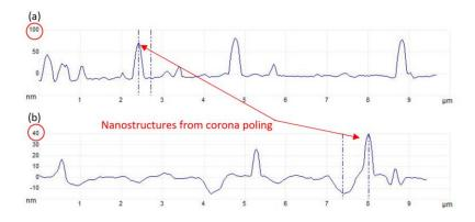
Figure 4.16. Profiles of a corona-poled azobenzene thin film (a) prior to and (b) after a 20-hour UV exposure. The UV exposure reduced the height of the nanostructures created by corona poling.
