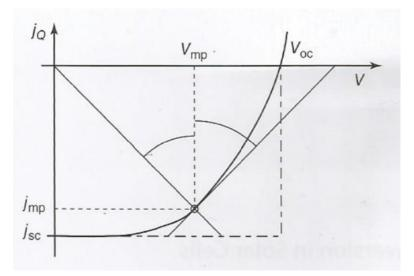
Figure 2.10. Geometrical construction of the maximum power point of a solar cell. The maximum power point occurs when the tangent to the characteristic J-V curve of a solar cell forms the same angle with a vertical line as the line connecting the origin to the maximum power point. Adapted from (Würfel and Würfel, 2016)<sup>1</sup>.
