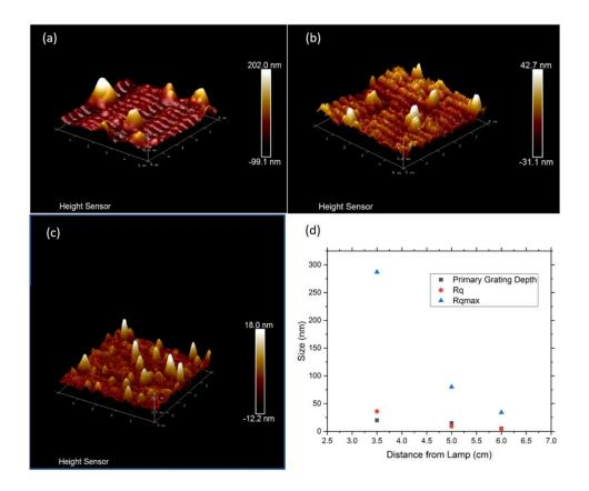
Figure 4.28. Effects of sample distance from the UV lamp on the size of the nanostructures. All three samples had identical original gratings and were exposed to UV light for 20 hours, with the distance to the lamp being (a) 3.5 cm, (b) 5 cm and (c) 6 cm.
