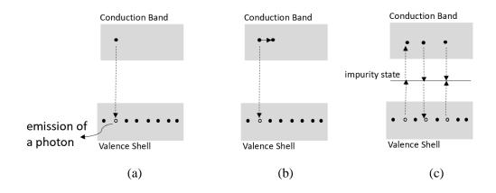
Figure 2.5. (a) Radiative, (b) Auger, and (c) SRH recombination. In (a), the energy from the recombination of the electron and hole is emitted in the form of a photon. In (b), the energy from the recombination is transferred to another electron. In (c), electrons and holes are trapped by impurities within the band gap.
