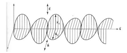
Figure 2.27. An electro-magnetic wave. In this graph, the magnetic field H is denoted as B. The electric field E, the magnetic field B, and wavevector k are mutually perpendicular. Adapted from (Pedrotti *et al.*, 2007)<sup>130</sup>.
