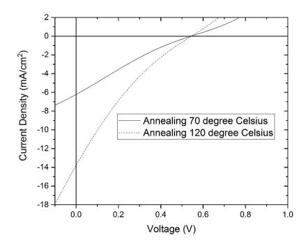
Figure 4.11. J-V characteristic curves of P3HT:PC<sub>61</sub>BM solar cells with low and high annealing temperatures. The low annealing solar cell exhibits a reduced  $J_{sc}$ .
