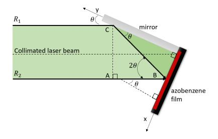
Figure 2.36. Top-view of the Lloyd's mirror interferometer. The mirror and sample form and angular angle of  $90^{\circ}$ . Half of the collimated laser bean illuminates the sample directly, while the other half is first reflected by the mirror, generating an optical path length difference and interference pattern.
