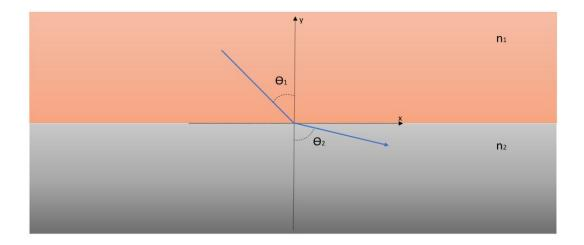
Figure 2.28. Refraction of a wave at the interface of two media with different index of refraction. In this case,  $n_1 < n_2$ .
