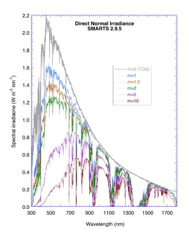
Figure 2.14. Irradiance spectra for increasing air mass. The solar radiation has been partially absorbed through its passage through the atmosphere in AM1 compared to AM0. AM1.5 shows even more absorption due to a longer path through the atmosphere. Adapted from (Wikipedia, 2013)<sup>86</sup>.
