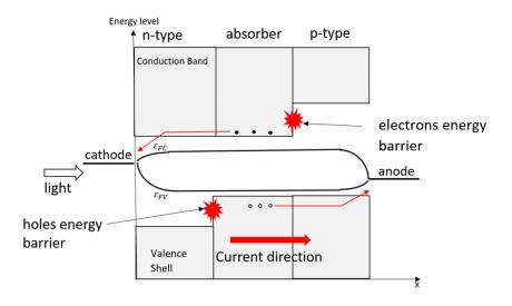
Figure 2.9. Quasi-Fermi levels in a pn-heterojunction. The differences in energy gaps of the material create energy barriers allowing only one type of carriers at the electrodes.
