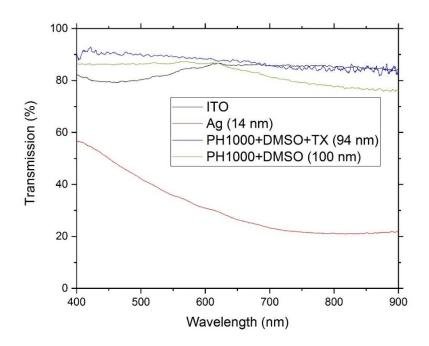
Figure 4.7. Transmission of ITO, PH1000 and Ag electrodes. While a  $\sim$ 100 nm PH1000 electrode is an acceptable alternative to ITO, a thin 14 nm layer of Ag without an anti-reflective coating has a significantly lower transmission in the visible range.
