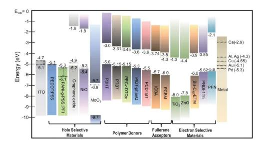
Figure 2.23. Energy levels of some common components used in organic solar cells. Adapted from (Yip and Jen, 2012)<sup>75</sup>.
