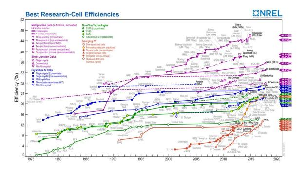
Figure 1.2. Best research solar cell efficiencies. The efficiency of conventional first-generation solar cell (in blue in the graph) has plateaued around 25%. Courtesy of the National Renewable Energy Laboratory, Golden, CO<sup>11</sup>.
