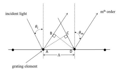
Figure 2.32. Light diffraction by two consecutive elements of a reflective grating elements separated by a distance  $\Lambda$ .
