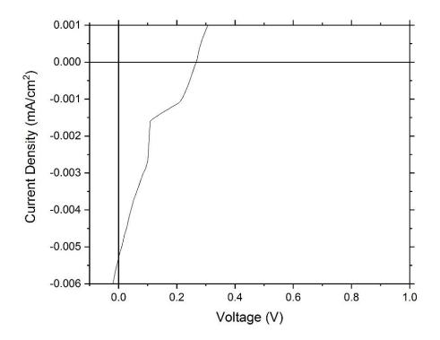
Figure 4.5. J-V characteristic curve of an inverted solar cell with a 14 nm Ag top electrode. This solar cell exhibited low  $R_{SH}$ ,  $J_{sc}$ ,  $V_{oc}$ , and FF.
