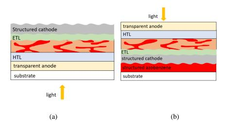
Figure 2.33. Organic solar cell structures for surface plasmons. For the direct structure in (a), the ETL can be patterned using a PDMS stamp before evaporation of the cathode. For the inverted structure in (b), a layer of azobenzene can be patterned via laser lithography before deposition of the cathode.
