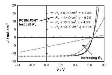
Figure 2.12. Modeled effect of  $R_S$  variation on the J-V characteristics of a P3HT:PC<sub>61</sub>BM cell. An increase in  $R_S$  results a decrease in FF, current density and efficiency. Adapted from (Servaites *et al.*,2010)<sup>77</sup>.
