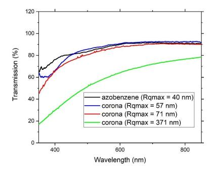
Figure 4.23. Transmission of azobenzene thin films patterned by UV exposure only ( $R_{qmax} = 40$  nm) or a combination of corona poling and UV exposure ( $R_{qmax} = 57, 71, 371$  nm). While the UV exposure resulted in good transmission for wavelengths above 500 nm, the transmissions of the thin films were not ideal for shorter wavelengths. High values of  $R_{qmax}$  also resulted in poor transmission.
