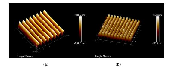
Figure 1.5. Atomic Force Microscope (AFM) images of (a) a linear grating and (b) a crossed grating.
