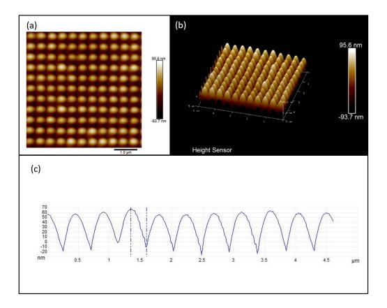
Figure 3.17. AFM (a) 2D image, (b) 3D image and (c) profile of a crossed grating on an azobenzene thin film. Parameters were laser irradiance of 416 mW/cm<sup>2</sup>, grating spacings of 450 nm and exposure times of 120 s and 55 s.
