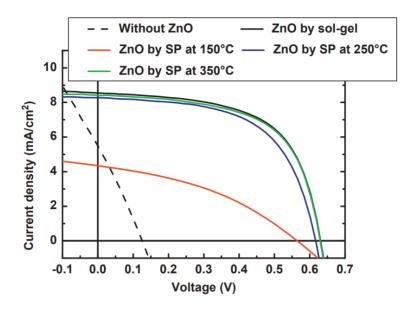
Figure 4.6. J-V characteristic curves of P3HT:PC<sub>61</sub>BM solar cells with and without ZnO. The solar cell without a ZnO ETL displayed low  $R_{SH}$ ,  $J_{sc}$ ,  $V_{oc}$ , and FF. Adapted from (Noh *et al.*, 2013)<sup>175</sup>.
