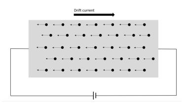
Figure 2.7. Drift current in a semiconductor. The direction of the drift current depends on the polarity of the applied electrical field.
