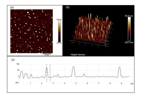
Figure 3.18. AFM (a) 2D image, (b) 3D image and (c) profile of nanostructures fabricated by corona poling of an azobenzene thin film heated at 75°C. An exposure time of 30 minutes and discharge voltage of 8 kV were used.
