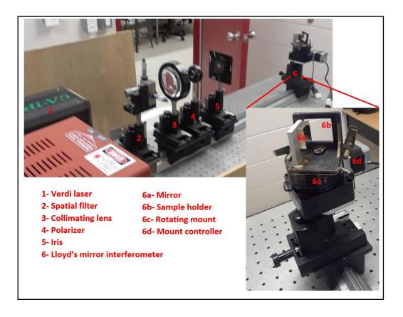
Figure 3.2. Surface relief grating station. This set-up was used to write SRGs on azobenzene thin films. The Lloyd's mirror interferometer is detailed in the inset.
