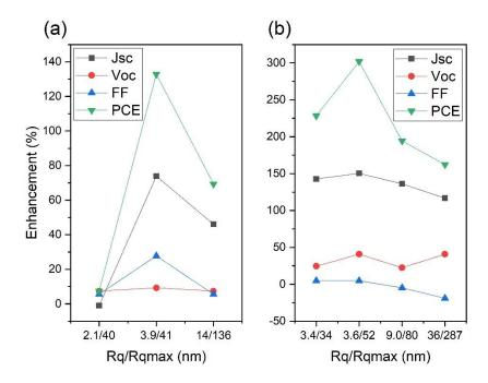
Figure 4.33. Enhancements of the solar cells characteristics of (a) P3HT:PC<sub>61</sub>BM and (b) PTB7:PC<sub>61</sub>BM solar cells after incorporation of azobenzene thin films patterned by crossed gratings and UV exposure. An improved  $J_{sc}$  and PCE are observed, with optimal values achieved with increased  $R_q$  as long as the  $R_{qmax}$  remained below ~ 60 nm.
