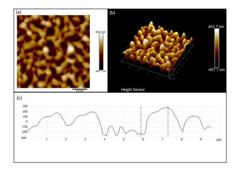
Figure 3.19. AFM (a) 2D image, (b) 3D image and (c) profile of a nanostructures fabricated by corona poling of an azobenzene thin film heated at 80°C. An exposure time of 30 minutes and discharge voltage of 8 kV were used.
