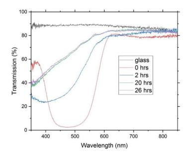
Figure 3.21. Transmission of an azobenzene thin film after UV exposure. The black line represents the transmission of glass only, and the color lines are the transmission of the azobenzene film and its glass substrate after different exposure times. The transmission saturated after a 20-hour exposure.
