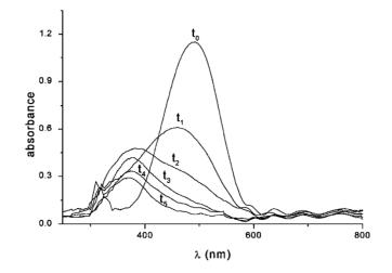
Figure 2.43. Evolution of the absorption spectrum of an DR1 azobenzene thin film upon 488 nm, 20 W/cm<sup>2</sup> irradiation. t<sub>0</sub>, t<sub>1</sub>, t<sub>2</sub>, t<sub>3</sub>, t<sub>4</sub> and t<sub>5</sub> correspond to irradiation times of 0, 5 minutes, 20 minutes, 60 minutes, 2 hours and 20 hours respectively. Adapted from (Galvan-Gonzalez *et al.*, 1999)<sup>148</sup>.
