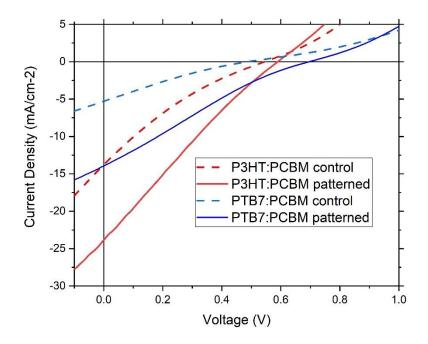
Figure 4.34. J-V characteristic curves of the best P3HT:PC $_{61}BM$  and PTB7:PC $_{71}BM$  solar cells with azobenzene thin film patterned by crossed gratings and UV exposure. PCE) enhancements of 133% and 302% compared to control solar cells were achieved for P3HT:PC $_{61}BM$  and PTB7:PC $_{61}BM$  solar cells, respectively.
