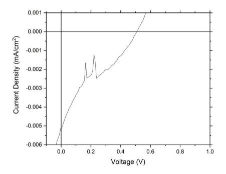
Figure 4.8. J-V characteristic curve of an inverted solar cell with a PH1000 top electrode. This solar cell displayed low  $R_{SH}$  and  $J_{SC}$ .
