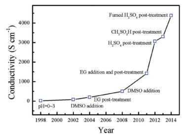
Figure 2.25. Timeline of PEDOT:PSS treatment aimed at improving its conductivity. Adapted from (Shi *et al.*, 2015)<sup>23</sup>.
