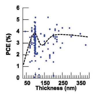
Figure 2.21. Efficiency as a function of P3HT:PC<sub>61</sub>BM active layer thickness. The dots represent the reported thickness and associated efficiencies. A thickness of 90 nm produces the maximum efficiency and has been the choice of several studies. Adapted from (Dang *et al.*, 2011)<sup>72</sup>.
