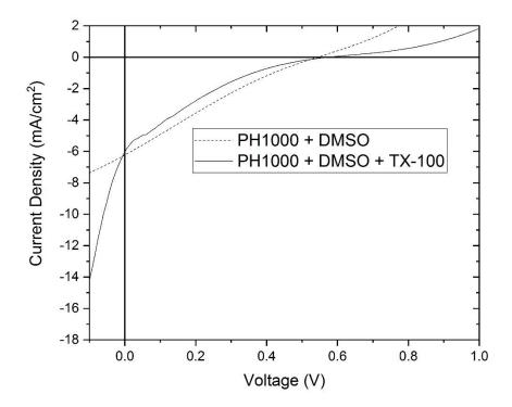
Figure 4.12. J-V characteristic curves of P3HT:PC<sub>61</sub>BM solar cells fabricated with bottom a PH1000 electrodes with and without the addition of surfactant. The addition of 0.5% wt TX-100 to the PH1000 solution had minimal impact on the parameters of the solar.
