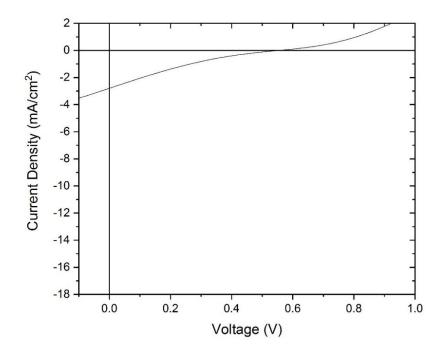
Figure 4.1. J-V characteristic curve of an ITO/Al 4083/P3HT:PC<sub>61</sub>BM/Al solar cell with an active area of 29.5mm<sup>2</sup>. This solar cell exhibited a good  $V_{oc}$ , but poor  $J_{sc}$ , FF and efficiency.
