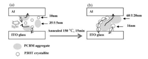
Figure 2.22. Schematic representation of P3HT:PC<sub>61</sub>BM blends a) in non-annealed solar cell and b) after annealing at 150°C for 15 minutes. The annealed device shows a good percolated network allowing for the passage of electrons and holes to the electrodes. Adapted from (Chiu *et al.*, 2008)<sup>107</sup>.
