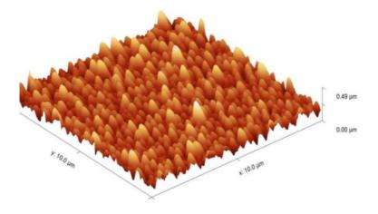
Figure 2.40. AFM scan of an electric-field-induced nanoscale surface patterning in azobenzene thin film. The film was exposed to an 8kV corona voltage at 80°C for 30 minutes. Adapted from (Umezawa *et al.*, 2016) <sup>67</sup>.
