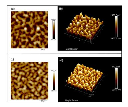
Figure 4.17. 2D and 3D images of large nanostructures on a corona-poled azobenzene thin film prior, (a) and (b), and after (c) and (d), a 20-hour UV exposure. The difference in the scales indicate a significant partial destruction of the nanostructures after UV exposure.
