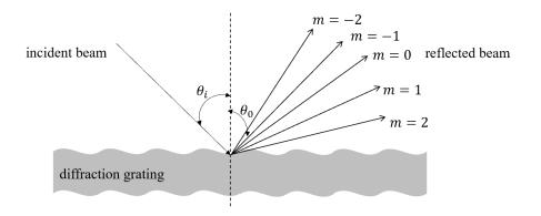
Figure 2.30. Diffraction of light with a reflective grating. The 0th order correspond to a reflection angle equal to the incident angle  $\theta_i = \theta_0$  (i.e. no diffraction).
