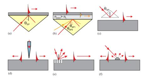
Figure 2.29. Surface plasmon excitation configurations. (a) Kretschmann geometry, (b) two-layer Kretschmann geometry, (c) Otto geometry, (d) excitation with a near-field scanning optical microscopy (SNOM) probe, (e) diffraction on a grating, and (f) diffraction on surface features. Adapted from (Zayats *et al.*, 2005)<sup>134</sup>.
