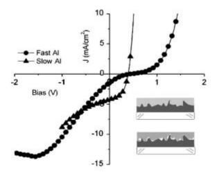
Figure 3.10. Effect of fast aluminium evaporation rate (200 nm/5 s) and slow evaporation rate (200 nm /100 s) on the J-V plot of a P3HT:PC<sub>61</sub>BM solar cell. The interface morphology is shown in the inset, with the slow evaporation at the top and the fast evaporation at the bottom. The fast evaporation creates voids at the interface, leading to a concavity of the J-V curve. Adapted from (Gupta *et al.*, 2010)<sup>162</sup>.
