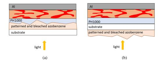
Figure 3.23. (a) Single-sided and (b) double-sided solar cells with patterned and bleached azobenzene thin films. The light is scattered by the patterned azobenzene films before entering the solar cells.
