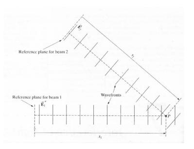
Figure 2.31. Two travelling plane waves interference, where  $s_1$  and  $s_2$  are the distances traveled by each beam from their sources to point P. Adapted from (Pedrotti *et al.*, 2007)<sup>130</sup>.
