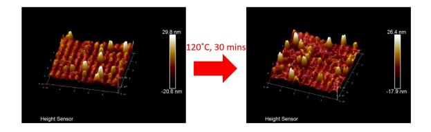
Figure 4.27. 3D Profile of a UV treated crossed grating on azobenzene thin film (a) before) and (b) after being heated at 120°C for 30 minutes. The high temperature exposure had no apparent effect on the nanostructures.
