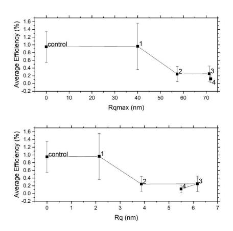
Figure 4.24. Average efficiencies of double-sided solar cells with patterned azobenzene thin films as a function of  $R_{qmax}$  and  $R_q$ . The solid lines are guides for the eyes only.
