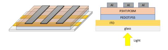
Figure 3.8. Schematic of direct structure ITO solar cell. This solar cell is a bottom-illuminated solar cell with an ITO layer as the anode, a PEDOT:PSS HTL, an active layer of P3HT:PC $_{61}$ BM blend and an aluminium cathode. The patterning of the electrodes produces six solar cells per sample, with the active area of the solar cell defined as the overlap of the electrodes.
