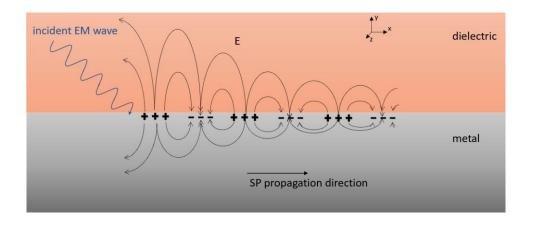
Figure 2.26. Surface plasmons schematic. The charge density oscillations induce an evanescent EM wave at the interface propagating in the *x*-direction and exponentially decaying in the *y*-direction.
