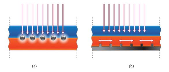
Figure 1.4. Plasmonic solar cells geometries. In (a), metallic nanoparticles act as subwavelength antennae to create a strong electric field near the nanoparticles, a phenomenon known as LSPR while in (b), the structured metal at the metal/absorber interface act as a light coupler to excite SPR, which results in an electrons wave propagating laterally in the cell. Adapted from (Atwater and Polman, 2010)<sup>36</sup>.
