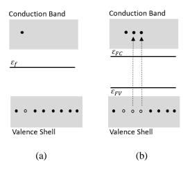
Figure 2.4. Quasi-Fermi levels for a semiconductor (a) in the dark and (b) illuminated. Under illumination, the absorption of the photons' energy causes the electrons to transition to the conduction band, increasing both the electron concentration in the conduction band and the hole concentration in the valence shell.
