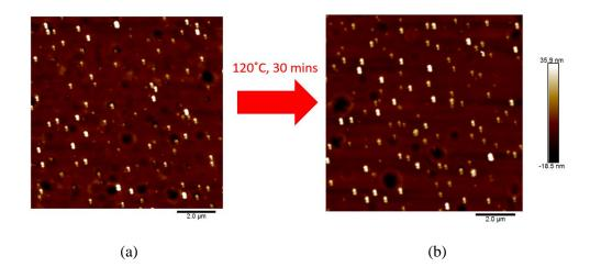
Figure 4.21. 2D profile of a corona-poled and UV treated azobenzene thin film (a) before and (b) after being heated at  $120^{\circ}$ C for 30 minutes. The high temperature exposure had no apparent effect on the nanostructures.
