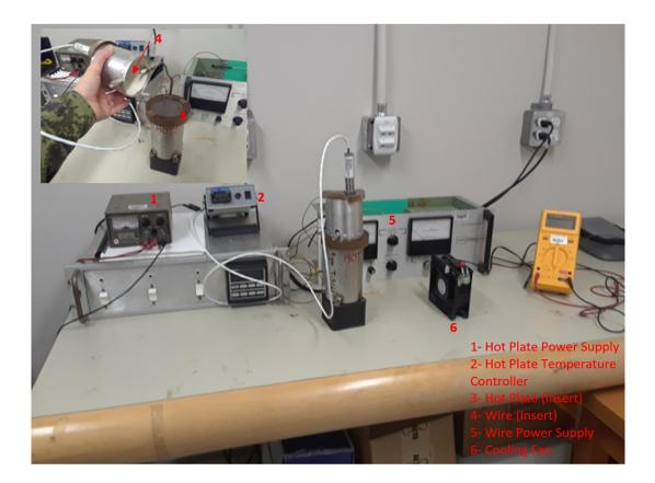
Figure 3.3. Corona poling set-up. The inset shows the wire suspended above the electrical hot plate.
