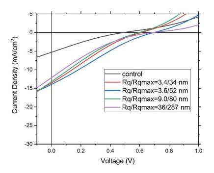
Figure 4.32. J-V characteristics curves for double-sided PTB7:  $PC_{61}BM$  solar cells with azobenzene thin films patterned by crossed gratings and UV exposure. As PTB7 solar cells are less susceptible to the transmission of azobenzene thin films than P3HT solar cells, the PTB7 patterned solar cells exhibited stronger efficiency enhancements than the P3HT solar cells.
