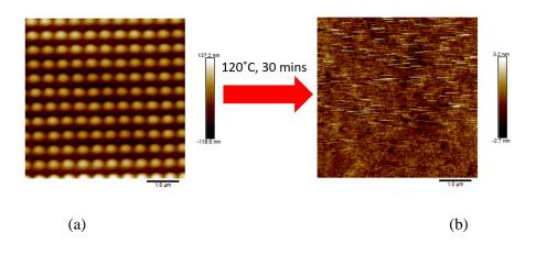
Figure 4.25. 2D profile of a crossed grating on an azobenzene thin film (a) prior to and (b) after heating at 120°C for 30 minutes. Heating the azobenzene thin film above its glass transition temperature erased the grating.
